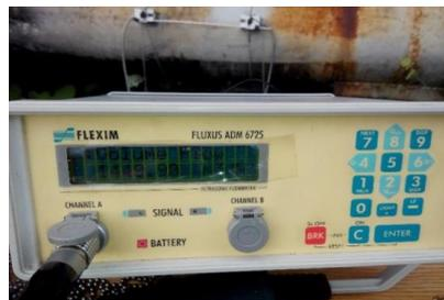
**Fig. 3.** Ultrasonic flowmeter recording a flow rate of 1449,90 m<sup>3</sup>/h
