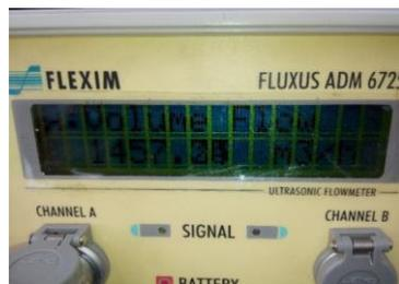
**Fig. 5.** Ultrasonic flowmeter recording a flow rate of 1457,33 m<sup>3</sup>/h.
