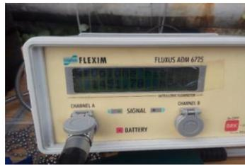
**Fig. 4.** Ultrasonic flowmeter recording a flow rate of 1451,78 m<sup>3</sup>/h.
